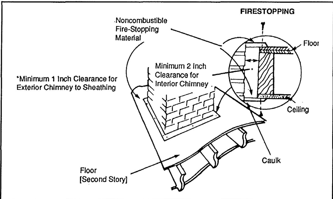
Remember that insulation must not contact the chimney. There must be an air space around the chimney and any insulation must be at least 2 in. or more from the chimney.
