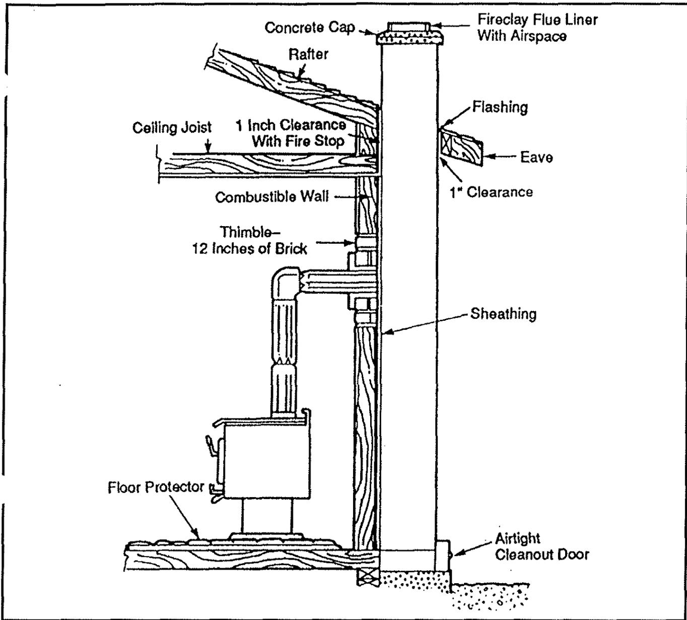
**2. 6 in. solid pack chimney with metal supports as a thimble** -- For the method of installation to a masonry chimney shown, it will be necessary to purchase a 8 in. inside diameter 12 in. long section of prefabricated listed solid chimney to use a thimble. Purchase a wall spacer, trim collar and wall band that are manufactured to fit the chimney section you purchase.
