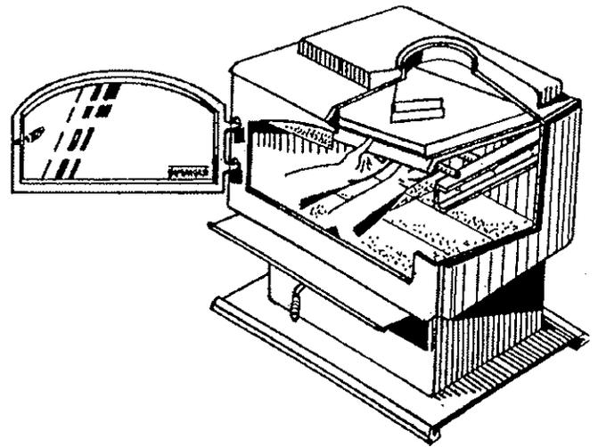
3. With a 3/16" Allen Wrench, remove the Secondary Combustion Tube Retainer Bolts on the Secondary Air Channel under the end of each tube. Note: Soak the bolts with penetrating oil at least 15 minutes before removal.
