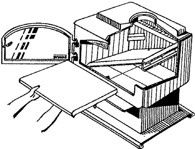
8. To replace the Baffle, reverse Steps 1 through 7. Be sure the stainless steel extension of the flame spreader is in place and resting on the Kaowool blanket. Be sure the hole in the rear of the Baffle is on the alignment pin.
