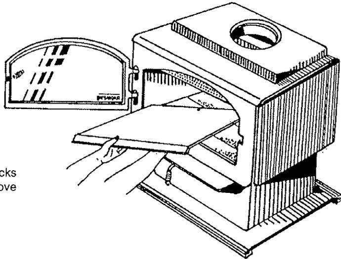
6. With one end of the Baffle resting on the bottom firebricks and the other end against the side of the Firebox, remove the Kaowool blanket.
