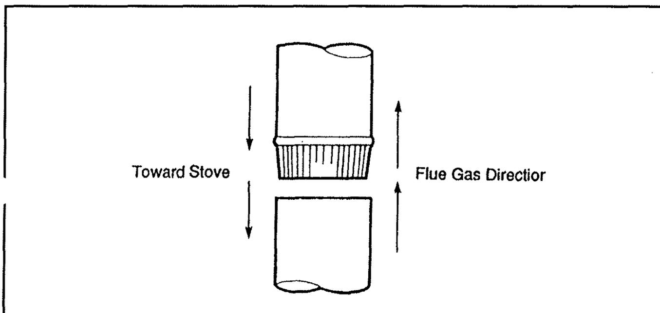
For proper operation the chimney connector should be as short as possible. Horizontal lengths of chimney connector should have a minimum upward slope from the stove of at least 1/4 in. per foot.
