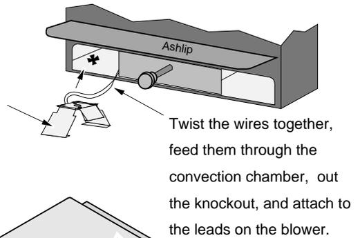
**f** Attach the blower to the stove with the three screws included with the blower.
