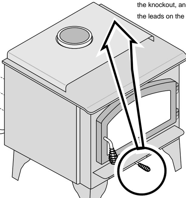
**g** Plug the blower in. Do not route the power cord under or over the stove or in a location where it may become damaged.
