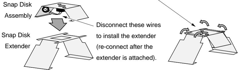
**c** Wedge the snap disk into the convection channel so. Bend the legs on the extender, if necessary, so the snap disk contacts the firebox.
