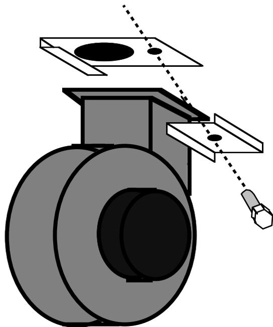
Once the convection fan is removed, place it so the impeller blades are facing up. Check the impeller blades for any damage and replace if necessary. Use a vacuum cleaner or brush to clean away any flyash that may have accumulated. Lubricate the convection fan bearings by dropping two drops of light machine oil into the two holes located on the outward side. Over-oiling can damage your fan.
