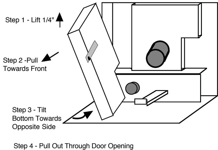
Remove the lower exhaust duct to complete the removal of internal firebox components.
