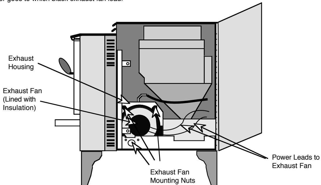
Once the exhaust fan is removed, place it so the side that holds the gasket is up. Check the impeller blades for any damage and replace if necessary. Use a vacuum cleaner or brush to clear away any flyash that may have accumulated. Lubricate the exhaust fan bearings located on both sides of the fan motor with two drops of light machine oil.
