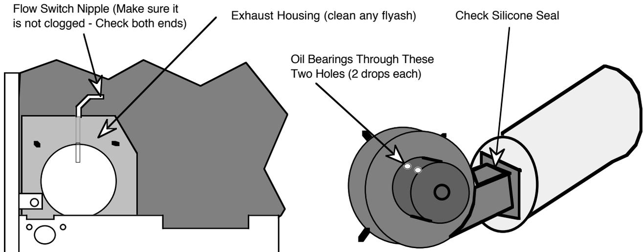
Prior to replacing the fan assembly, check that the silicone seal at the fan and exhaust tube. If fractured, use Type RTV 500 degree silicone sealant to reseal the joint.
