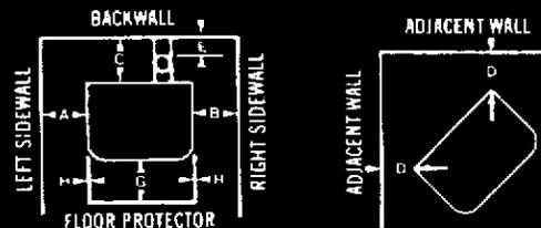
Maximum alcove depth 48 in./1220 mm, min ceiling height 60 in./1525 mm.
