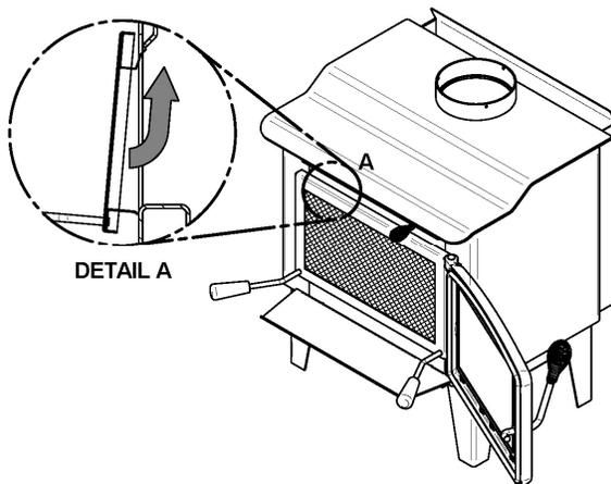
Lean the upper part of the fire screen against the top door opening making sure to insert the top fire screen brackets behind the primary air deflector as in (Detail A).
