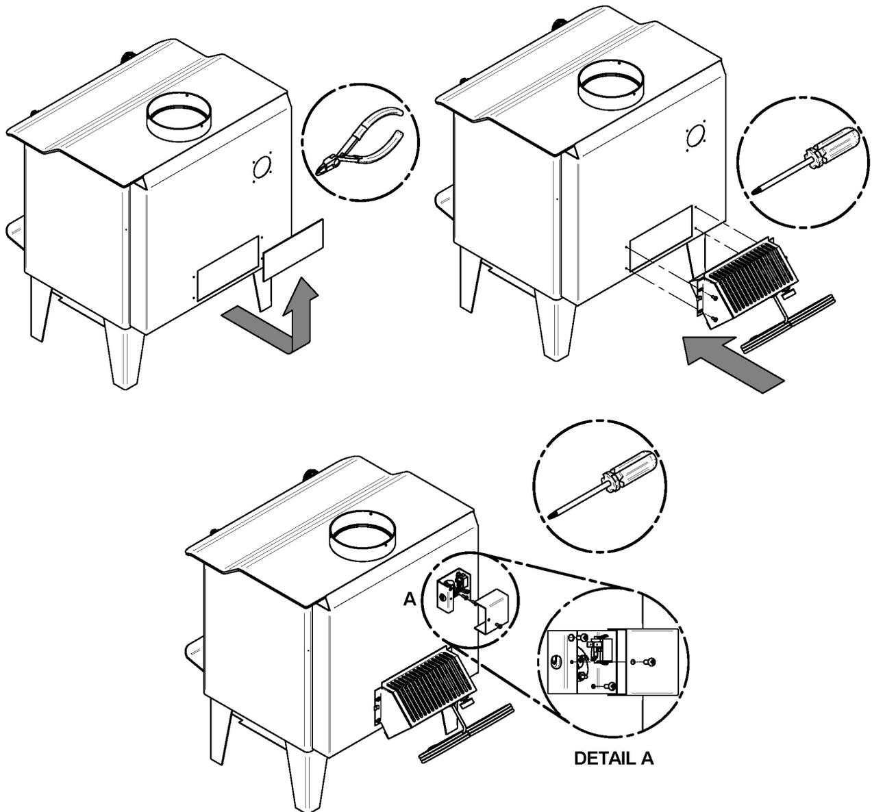
When using the optional blower, allow the stove to reach operating temperature (approximately one hour), before turning it on. The increased airflow from the blower cools the firebox and could affect the start-up combustion efficiency if the blower is turned on too early. You can also install a thermodisc to enable the blower to start or stop automatically when the stove is hot or too cold. The thermodisc kit part number is AC05530 for a basic model and ACO2055 for a quick connect model.
