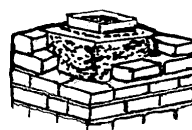
Tile-lined masonry chimney
