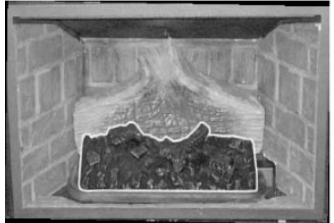
Figure 45: Place the ember bed in the center of the burner tube and pull it forward as far as it will go. Ensure it DOES NOT obstruct any part of the burner.
