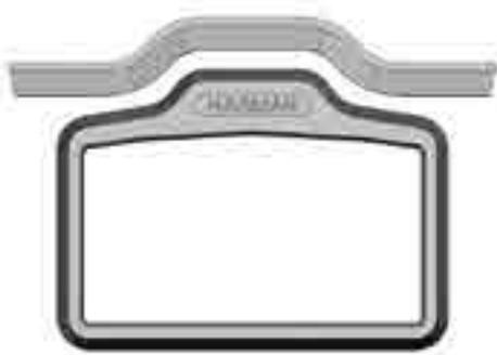
The coil spring handles slip onto the latches and the shaker handle. Push while turning to install.
