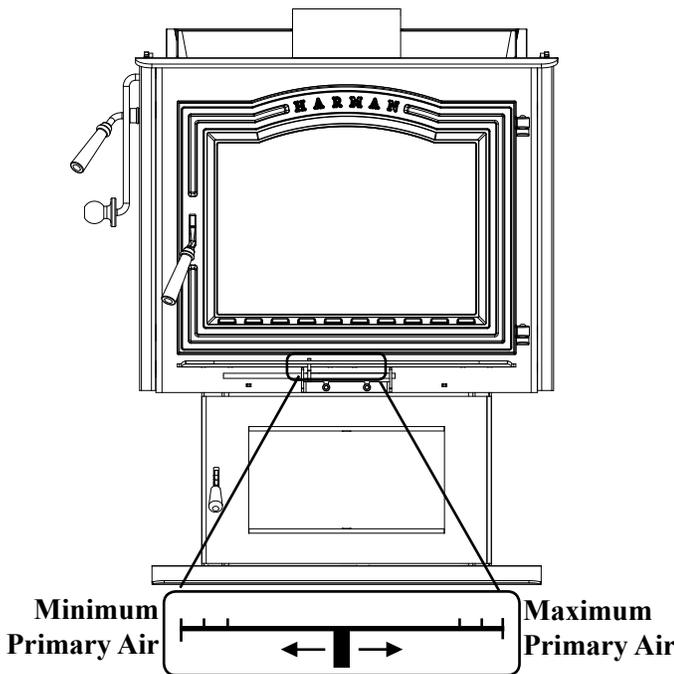
The air control lever is located on the ash lip, below the load door. Sliding this lever allows you to vary the amount of air to the fire, creating a range of heat outputs. The lowest heat output setting is to the left, and the highest is to the right. The notches are provided as a reference for your comfortable heat settings. Do not, under any circumstances, alter the configuration or operation of the air control lever.
