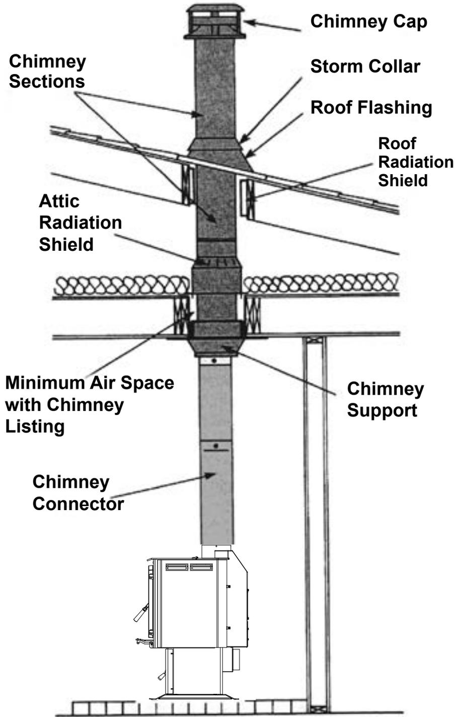
**The Chimney Connector Shall Not Pass Through an Attic or Roof Space, Closet or Similar Concealed Space, a Floor or Ceiling.**
