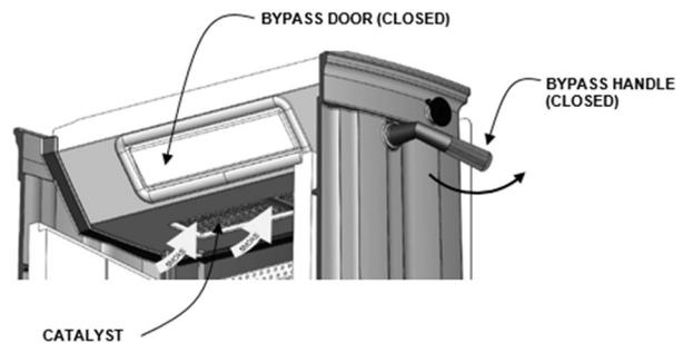
Figure 14 – Bypass Closed
