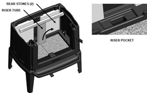
Figure 21 - Removing Riser and Rear Stones
