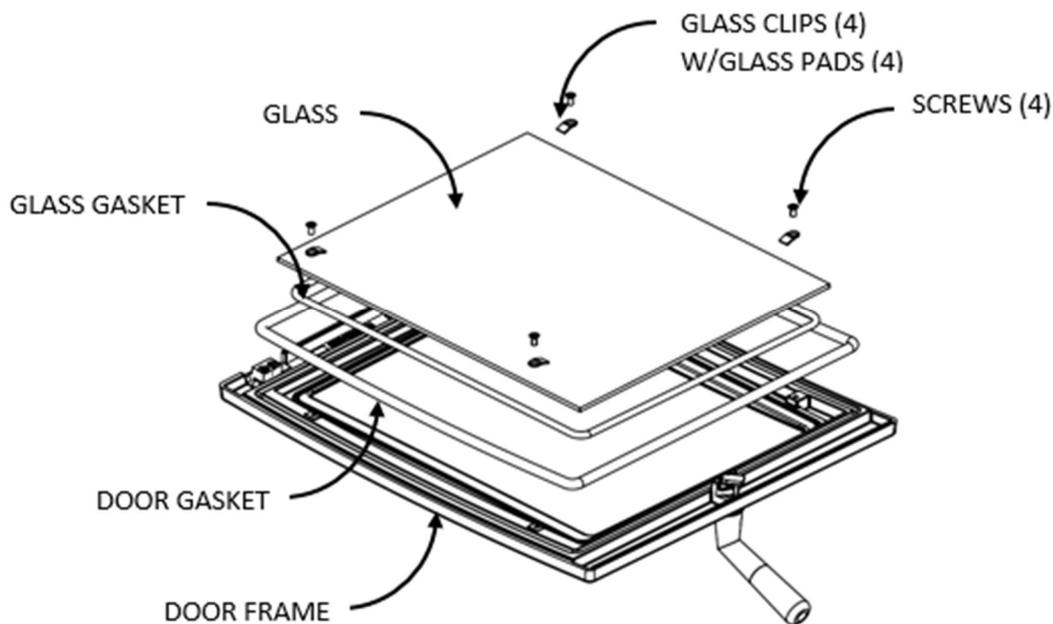
**Figure 22 - Front Door Assembly**
