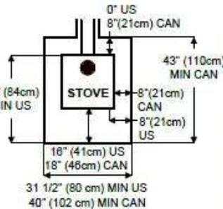
When installed on a combustible floor, non-combustible floor protection is required to cover the area beneath the heater, and extend at least 18" (46 cm) (18" (46 cm) CAN) to the front and 8" (21 cm) beyond each side of the fuel loading and ash removal openings (side of stove in CAN), the floor protection must extend under the flue connector and extend 2" beyond each side of pipe.
