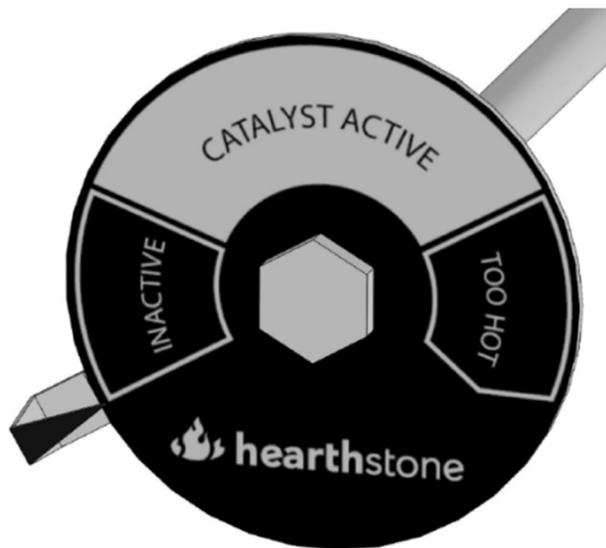
Figure 16 – Catalyst Thermometer
