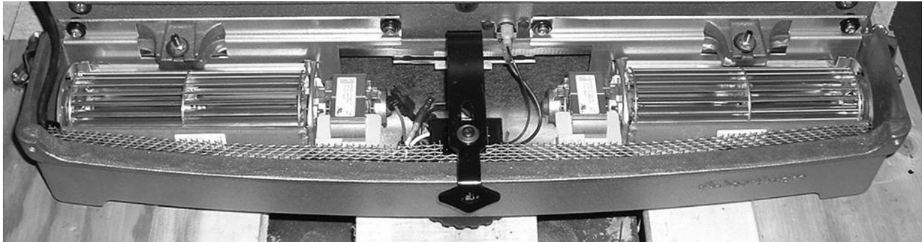
Photo 30 – Blower System (Ash Lip Cover Removed)
