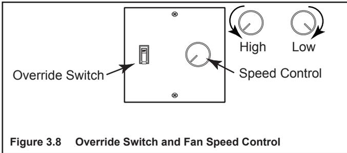
Figure 3.8 Override Switch and Fan Speed Control
