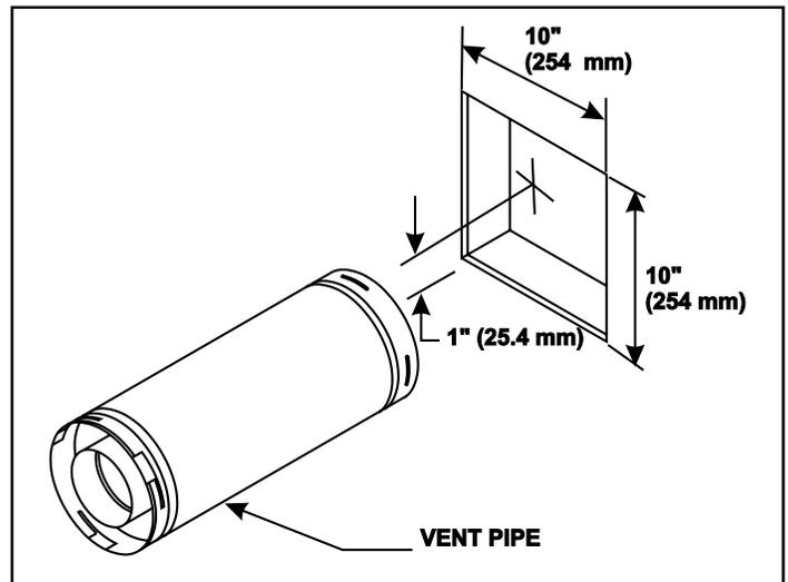
Figure 14. 10 in. X 10 in. Hole and Vent Pipe
