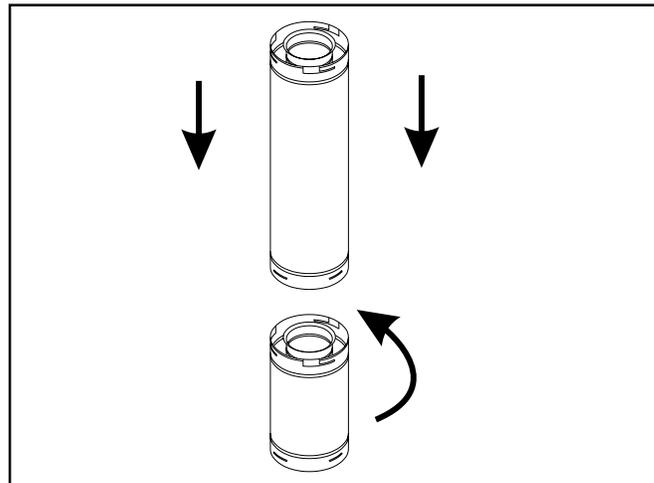
**Figure 12. Adding Venting Components**
