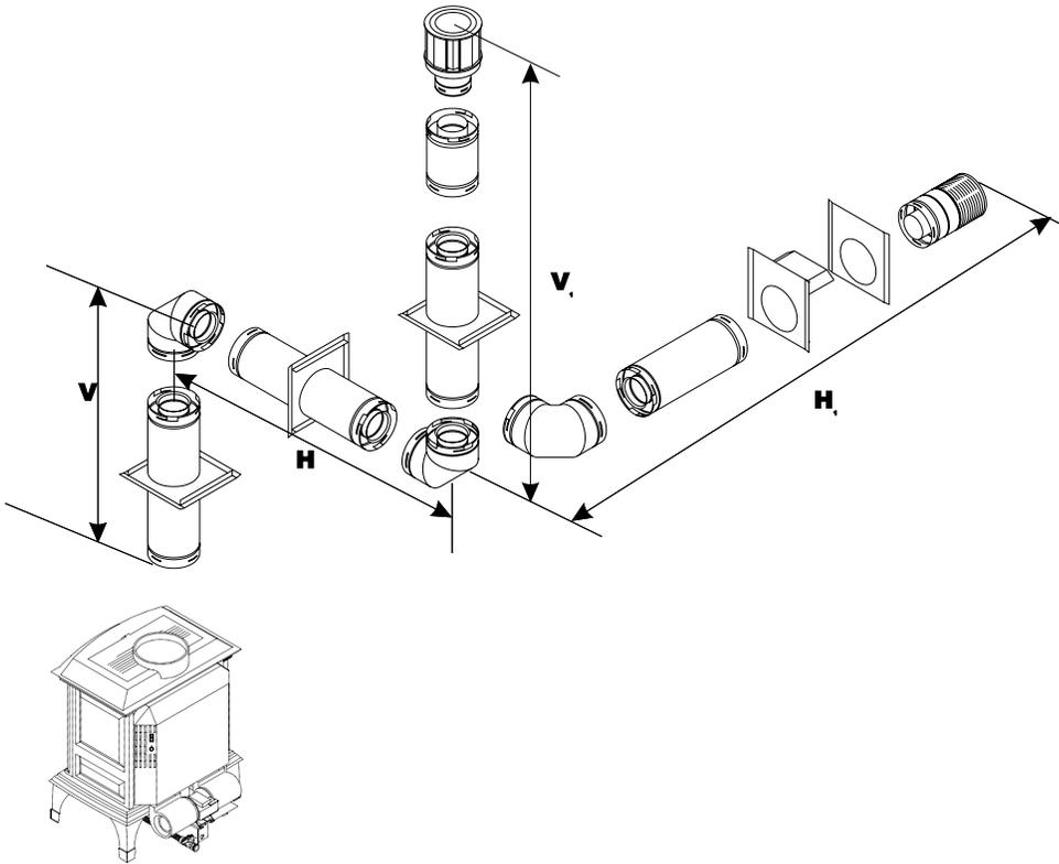
**Figure 9. Vent System with Two 90° Elbows**
