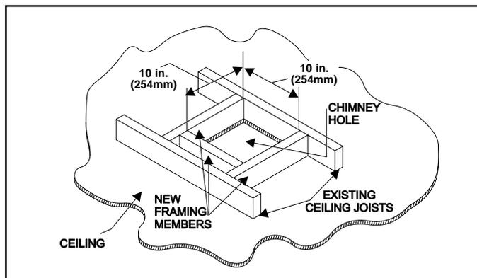
**Figure 16. 10" x 10" Hole and New Framing Members**
