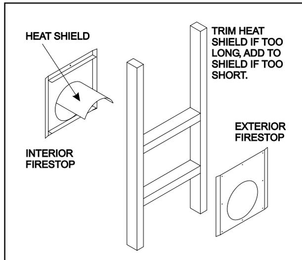
**Figure 15. Heat Shield, Interior and Exterior Firestops**
