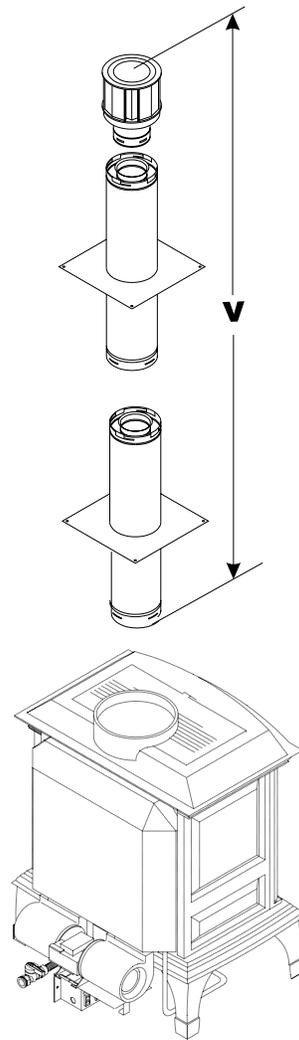
**Figure 7. Straight Vertical Vent System**
