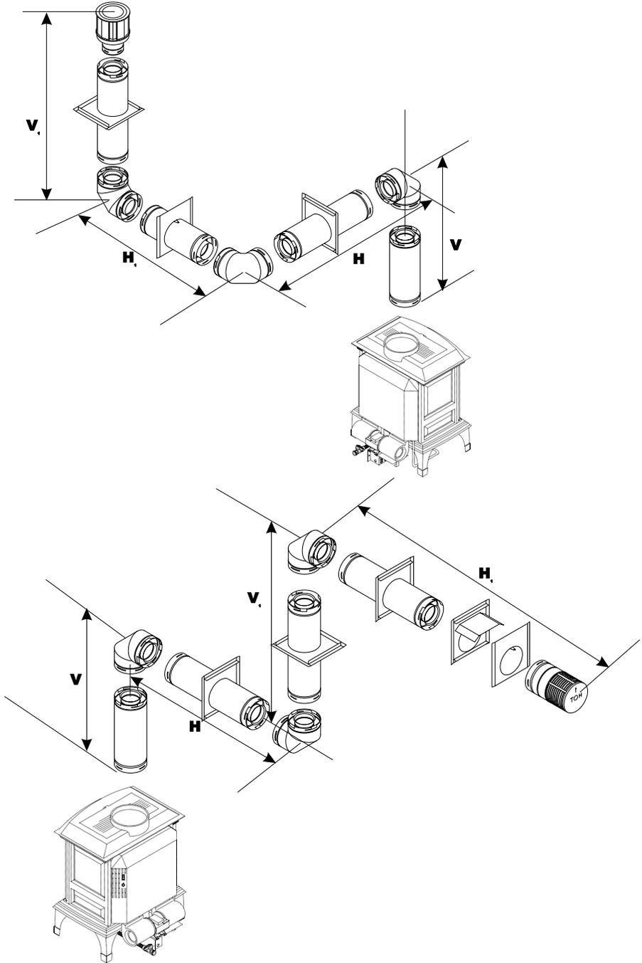
Figure 10. Vent System with three 90° elbows
