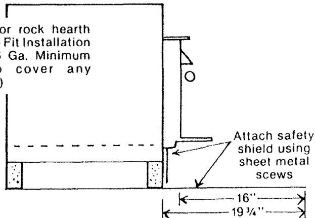
2. Set BUCKMATE unit in place and attach safety shield to unit as shown in Figure 1-A and 1-B. You must place a non-combustible material 3/4" thick millboard or equivalent K Factor = .084/BTU/F<sup>2</sup> H<sup>0</sup> F inches minimum. Note: 3/8" thick millboard may be used when installing the ZC-3-01 and 27000-B.
