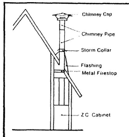
FIGURE 2 Through High Pitch Roof
