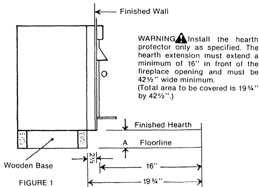
Base for BUCKMATE must be level with or slightly higher than finished hearth height - dimension (A) Figure 1. Front of BUCKMATE cabinet must be recessed 2 1/2" from finished wall.
