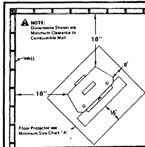
FIGURE 2 CORNER INSTALLATION
