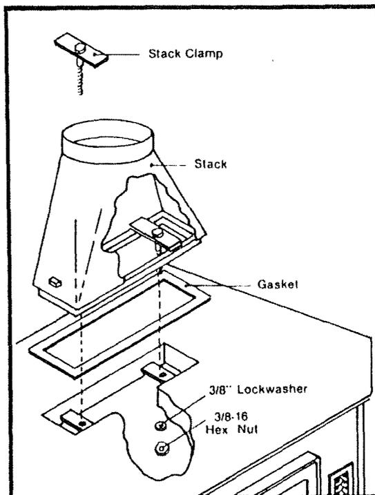
FIGURE 8 (MOUNTING STACK)
