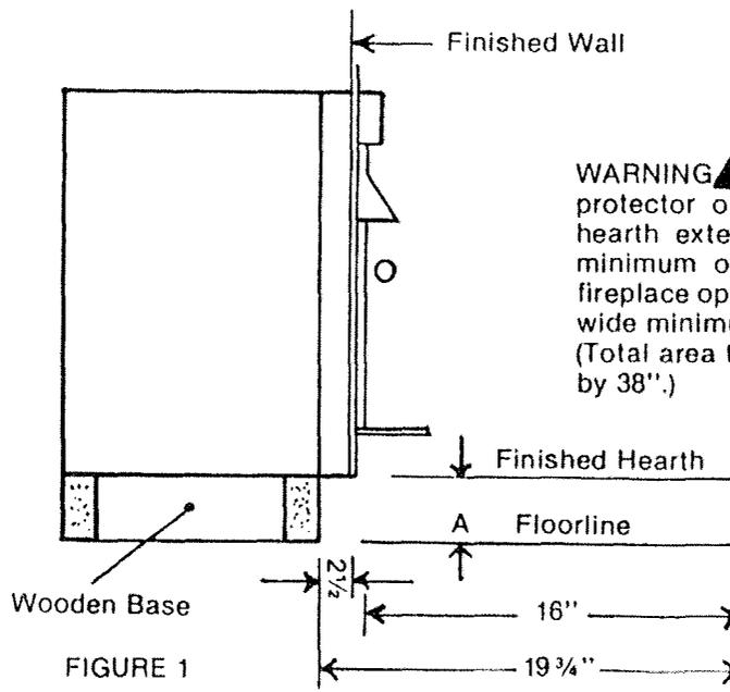
Base for BUCKMATE must be level with or slightly higher than finished hearth height - dimension (A) Figure 1. Front of BUCKMATE cabinet must be recessed 2 1/2" from finished wall.
