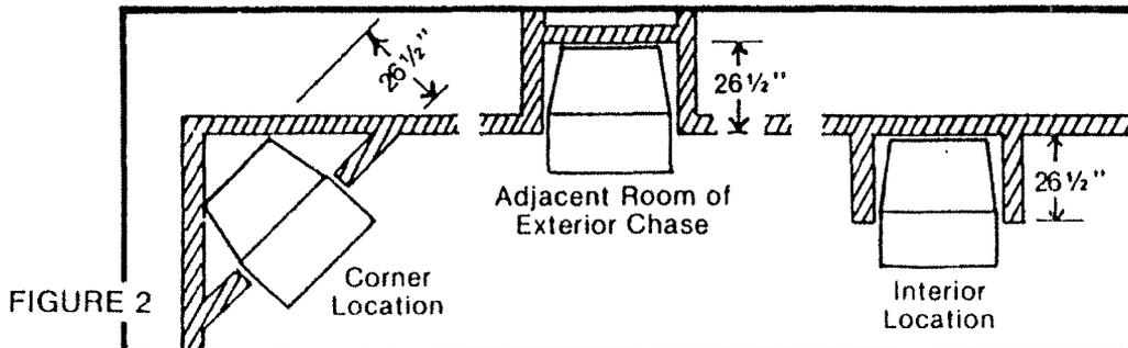
Above (Figure 2) are framing location examples with depth dimensions for some typical configurations. These are finished measurements so install accordingly.
