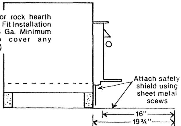
2. Set BUCKMATE unit in place and attach safety shield to unit as shown in Figure 1-A and 1-B. You must place a non-combustible material 3/8" thick millboard or equivalent .084K factor or 2" of masonry (brick or rock) over this area as a minimum.
