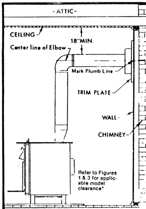
FIGURE 8 WALL CHIMNEY MOUNTING
