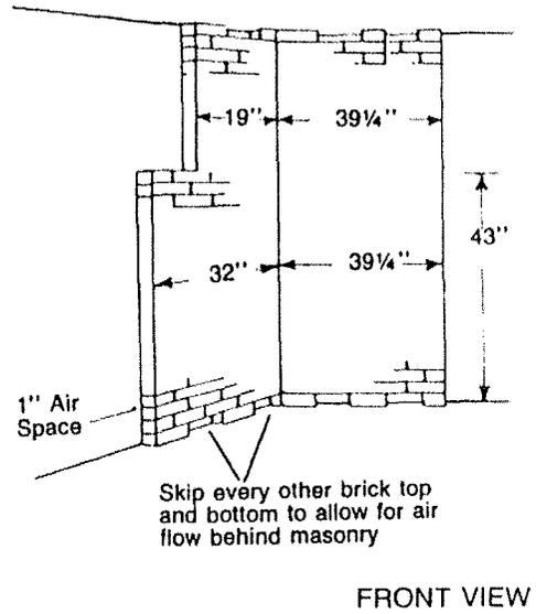
3. Using 24 ga. sheet metal with 1" ventilated air space.
