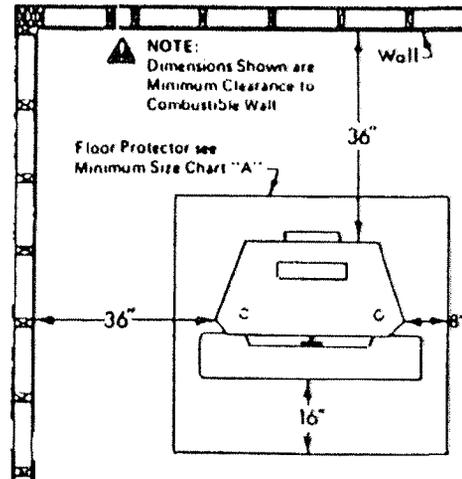
FIGURE 3 WALL INSTALLATION
