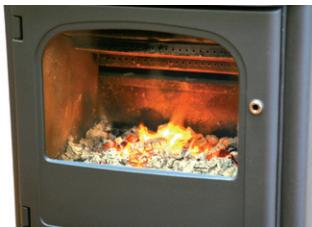
6. Place three pieces of fuel weighing roughly 0.6 kg and measuring about 25 cm in length across the embers in one layer, with spacing of roughly 1 cm between the pieces of wood.
