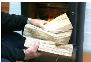
The stove door should normally be opened gently the first 2 - 3 centimetres, then you should wait until the pressure has equalised before opening the door all the way. This technique will prevent smoke from getting out, particularly when there is a poor draught.
