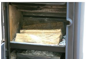
8. Once the new fuel has taken, adjust the secondary air amount to the desired setting; optimal combustion will continue until glowing charcoals are produced.
