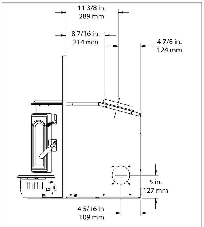
**Figure 31.4 - Side View Without Optional Flue Adapter**
