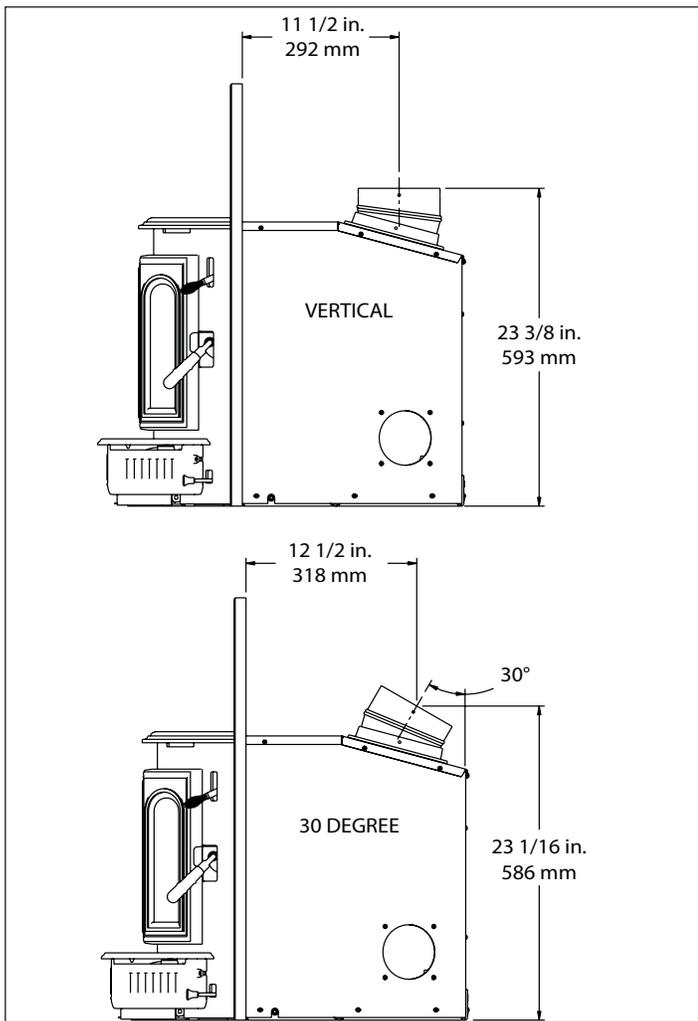
**Figure 31.3 - Side View With Optional Flue Adapter**
