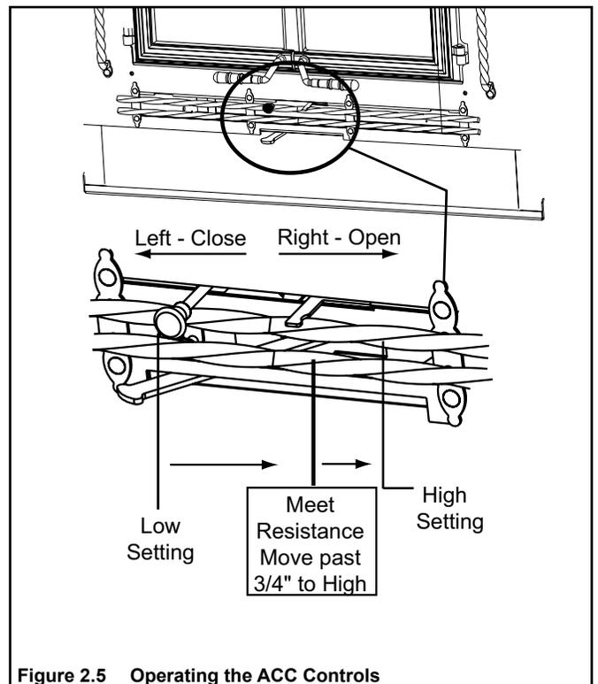
**Figure 2.5 Operating the ACC Controls**
