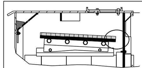
Ceramic Blanket and Baffle Board are **NOT** in contact with the back of the firebox.
