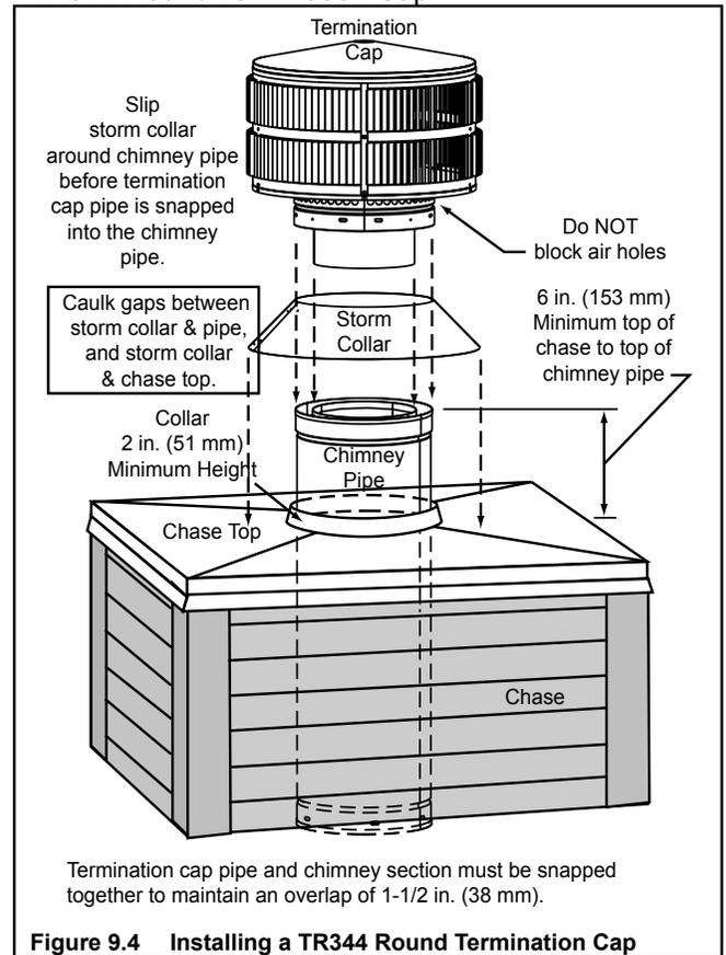
Figure 9.4 Installing a TR344 Round Termination Cap
