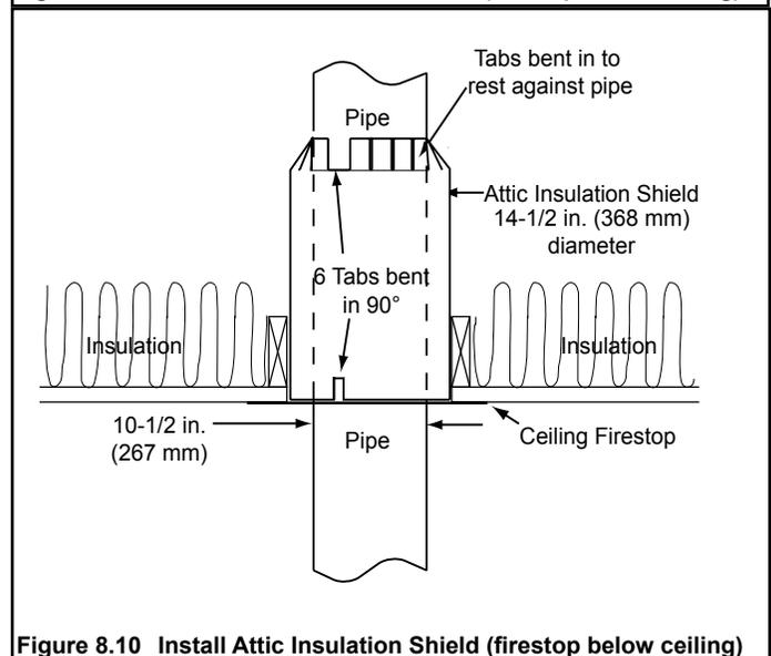
Figure 8.10 Install Attic Insulation Shield (firestop below ceiling)
