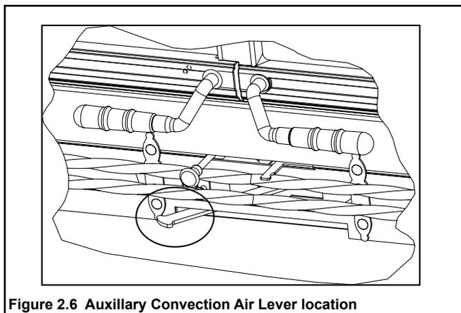
Figure 2.6 Auxiliary Convection Air Lever location
