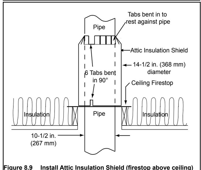
Figure 8.9 Install Attic Insulation Shield (firestop above ceiling)
