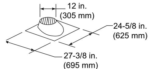
RF370 - Roof Flashing Flat to 6/12 Pitch
