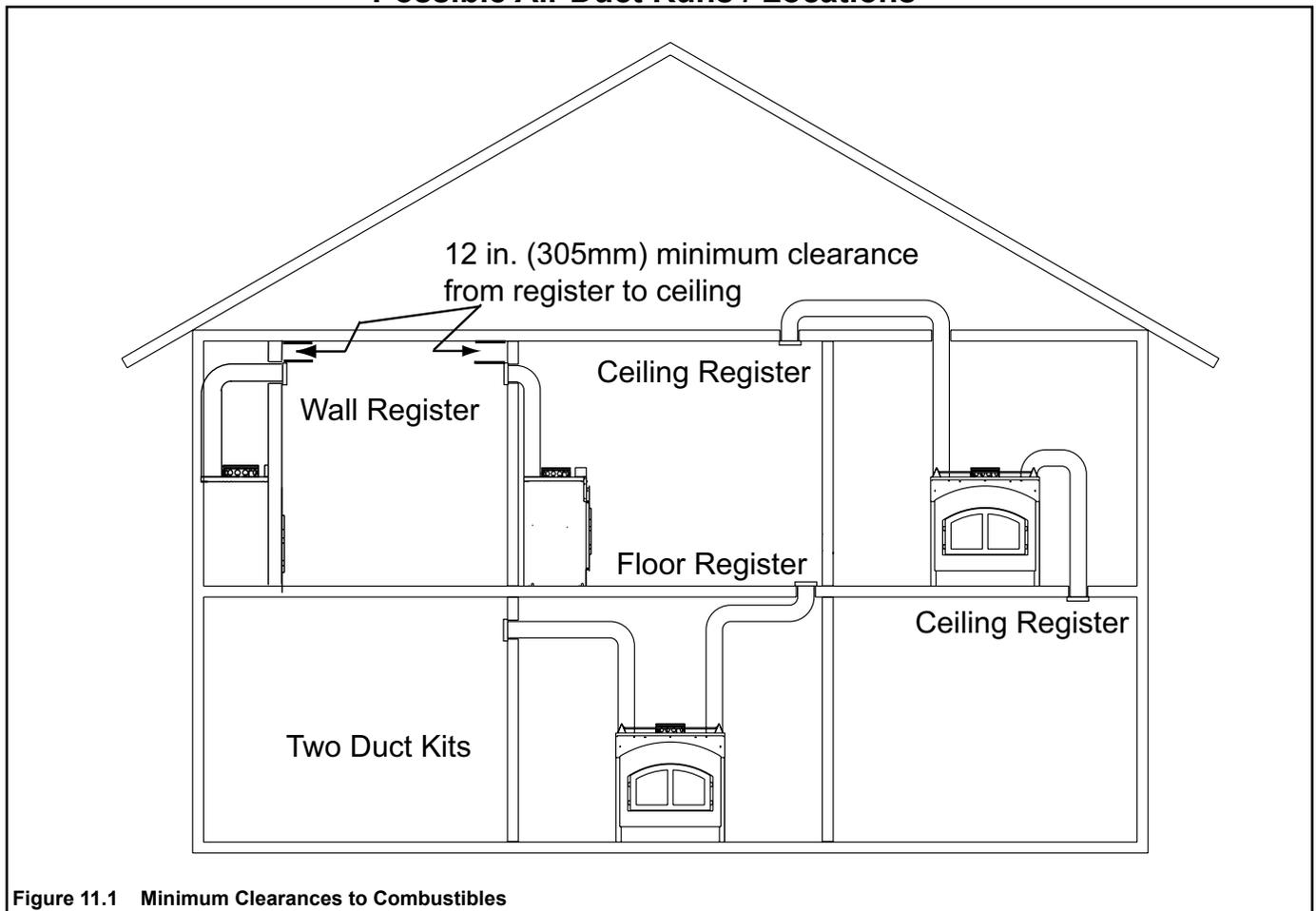
Figure 11.1 Minimum Clearances to Combustibles
