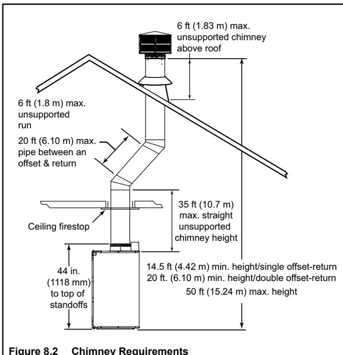
Figure 8.2 Chimney Requirements
