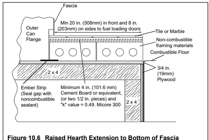
**Figure 10.6** Raised Hearth Extension to Bottom of Fascia
