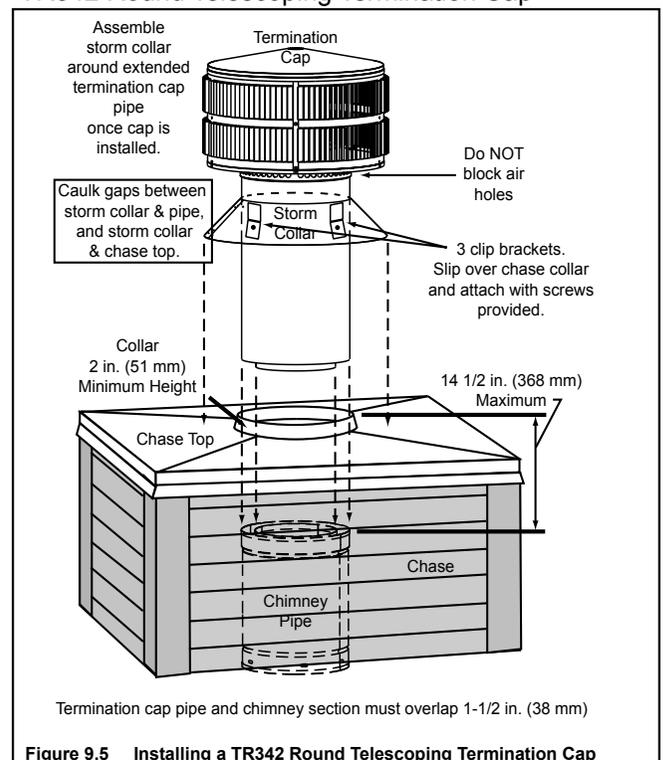
Figure 9.5 Installing a TR342 Round Telescoping Termination Cap
