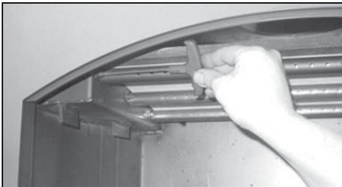
Figure 4.6 Removing Manifold Tube
