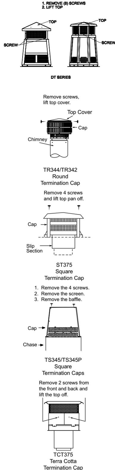
Figure 4.1 Chimney & Termination Cap Cleaning
