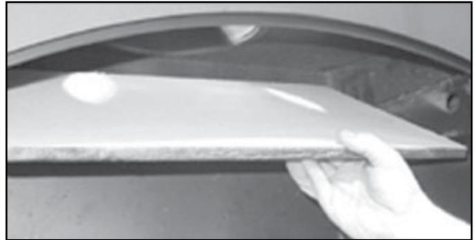
Figure 4.7 Removing Baffle (shown without ceramic blanket)
