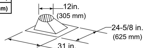
RF371 - Roof Flashing 6/12 to 12/12 Pitch
