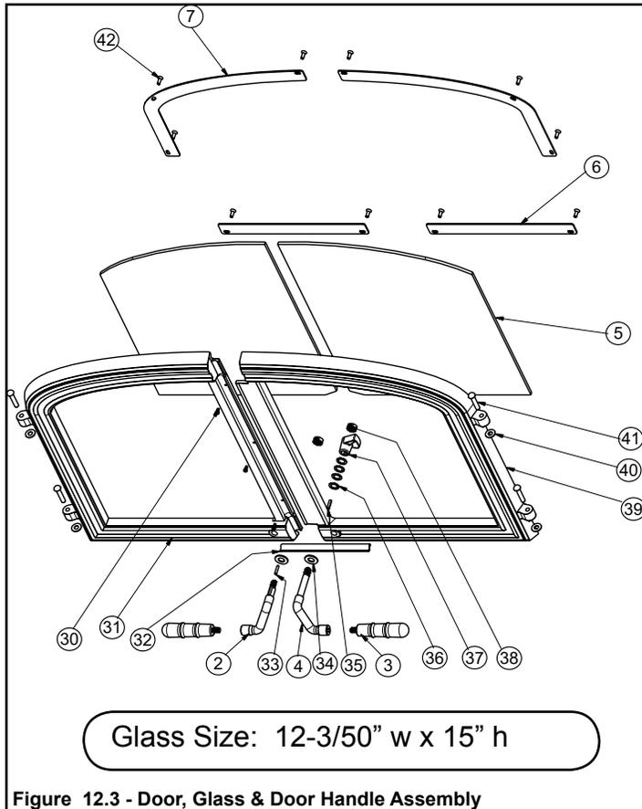
Figure 12.3 - Door, Glass & Door Handle Assembly
