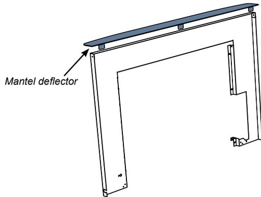
2. Bend all 3 tabs 90° to secure the deflector to the top of the backing plate. The tabs should be flush with the underside of the top lip of the back plate.
