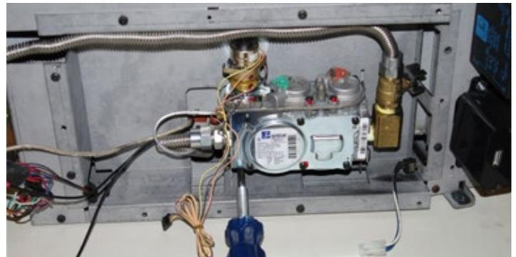
8) Remove the Gas Valve by lifting upwards and outwards.
