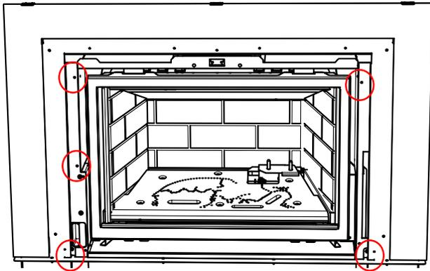
3. Attach the backing plate to the outer faceplate from the front with 7 screws (3 along the top and 2 on each side).
