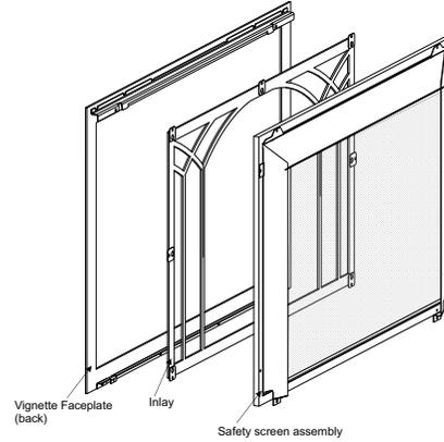
2. Remove 4 screws from the back of the Vignette faceplate in locations shown below—to remove the safety screen assembly.
