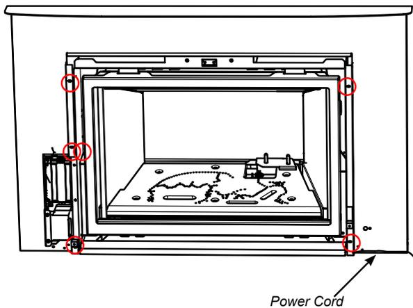
4. Install front faceplate by hooking back of front faceplate over lip edge on unit in locations shown below. Angle faceplate slightly to hook on, lower gently, bottom of faceplate will secure with magnets.
