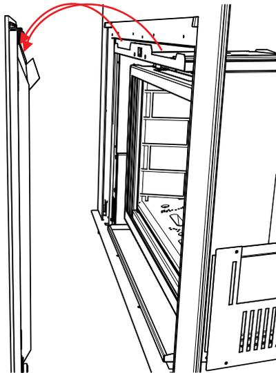
2. Remove the outer faceplate by removing the 5 screws as shown.
