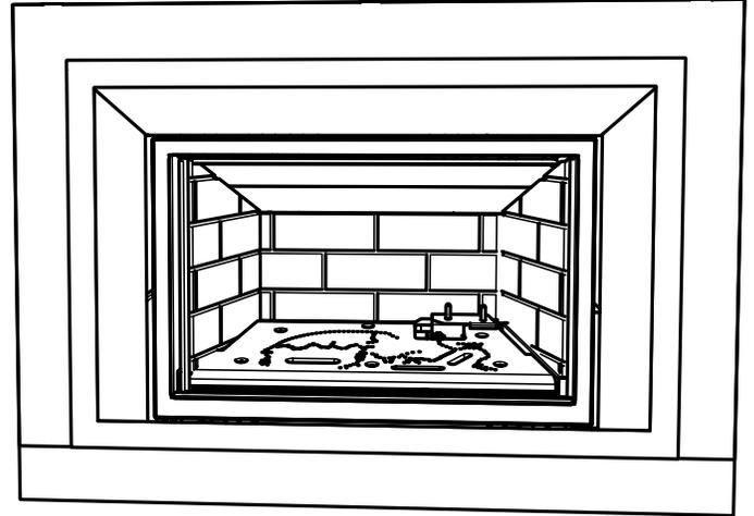
2. Install the outer faceplate by hooking the flange over the hanger as shown.
