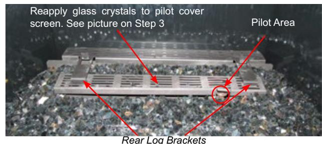
3. Place Log 1 on Rear Log Bracket in front of tabs, ensure Log is centered. Place small amount of glass crystals on pilot cover, over top pilot area in front of Log 1.
