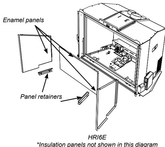
3. Install the firebox liner Left, with the corresponding Insulation Panel by sliding it into the left side of the firebox. The rear flange of the liner must fit between the firebox liner rear and the firebox. You may have to push the liner against the firebox as you push it rearward.
