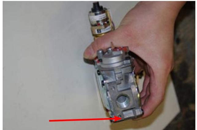
12) Place the Gas Valve into the machine vice using the provision as described above. Do not over tighten the vice. Remove the Flare Fitting from the gas outlet side of the valve.
