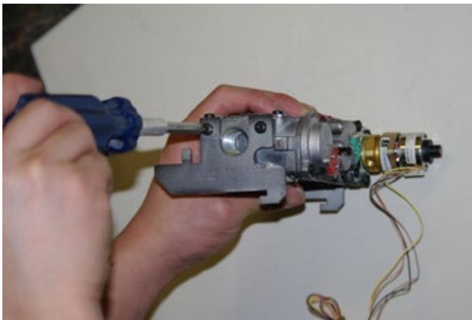
11) There is a provision in the Valve body casting that is designed to be used as a gripping point for assembly with other components. This is the portion of the valve that can be placed in a machine vice.
