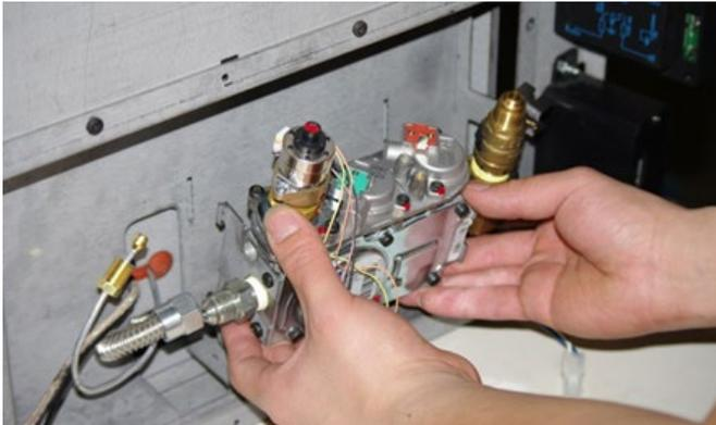
9) Secure the Valve Assembly by the 90 Elbow Fitting in a sturdy table vice. Using a crescent wrench, loosen the valve from the Elbow fitting.
