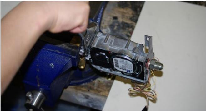
10) Remove the 2 screws that hold the Right Side Valve Mounting Bracket onto the Valve.
