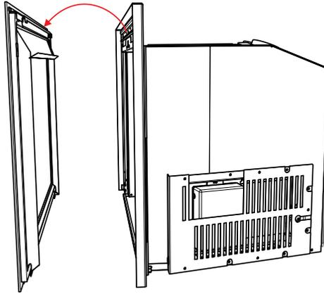
3. Position the inlay face down on the back of the Vignette faceplate and reinstall the safety screen assembly (reverse Step 2).
