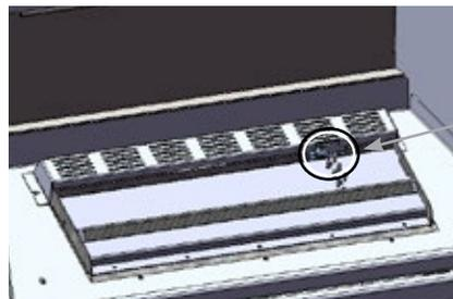
**Important:** Do not to install glass or other media in this area, as this will block the path of the pilot to the burner.
