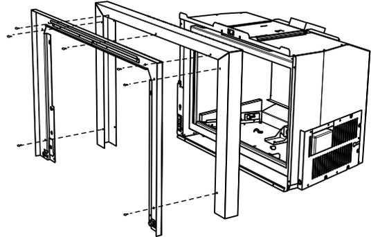
5. Reinstall the outer faceplate and spacer—reverse Step 2.
