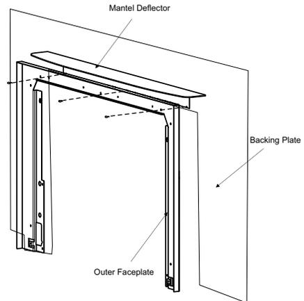
5. Reinstall the outer faceplate and spacer—reverse Step 2.
