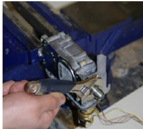
13) Remove the 2 screws that secure the left side valve mounting bracket from the gas valve.
