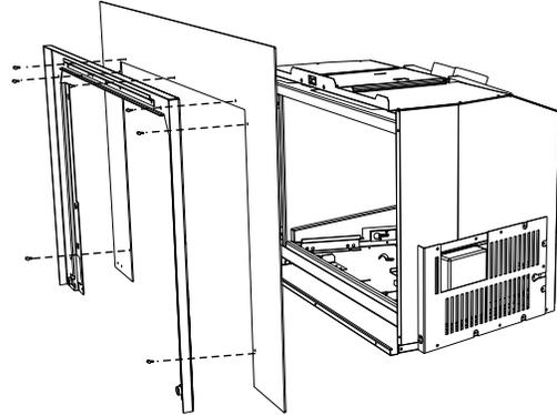
4. Reinstall the outer faceplate and backing plate—reverse Step 2.
