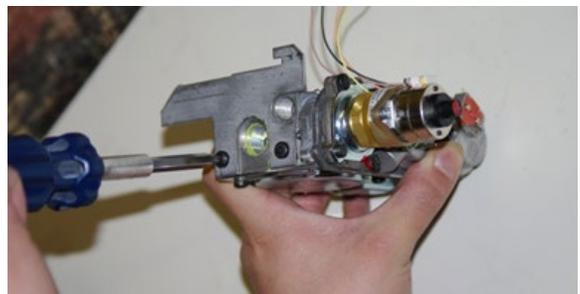
14) Replace the gas valve with the new unit and re-assemble by reversing disassembly steps 2-13.
