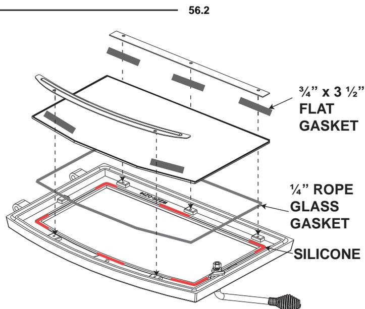
**NOTE:** For replacement glass, size, thickness and specifications see "REPLACEMENTS" section.
