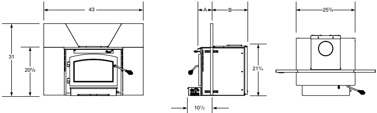
\* A and B are adjustable in 3/8" increments (see min max below).
