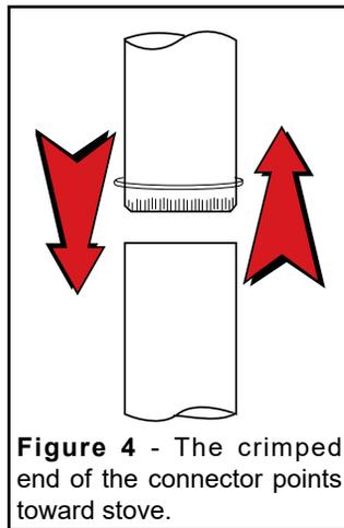
**Figure 4** - The crimped end of the connector points toward stove.
