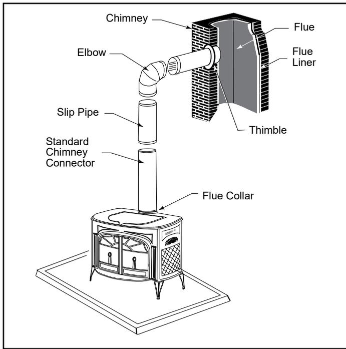
**Figure 6** - Chimney connection in a freestanding installation.
