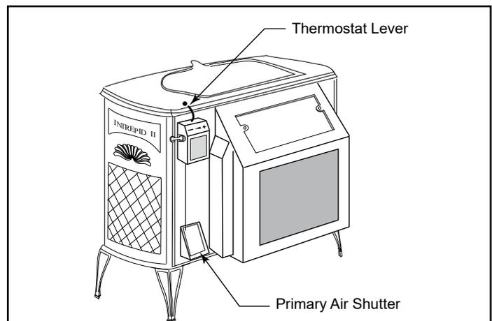
Figure 43 - The primary air shutter must move freely.
