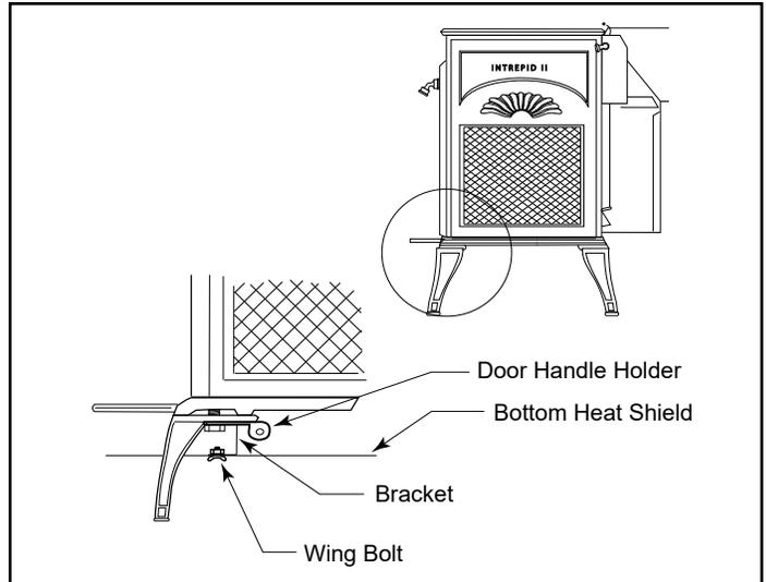
Figure 28 - Handle holder and heat shield positions.
