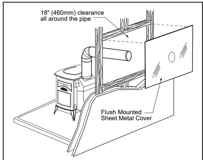
**Figure 10** - An approved wall pass-through for Canada.
