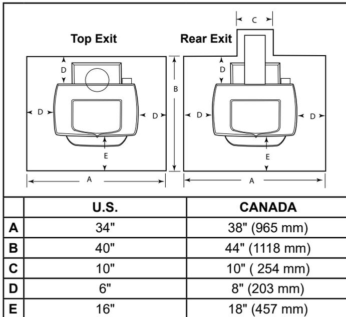
**Figure 11** - Required floor protector dimensions.
