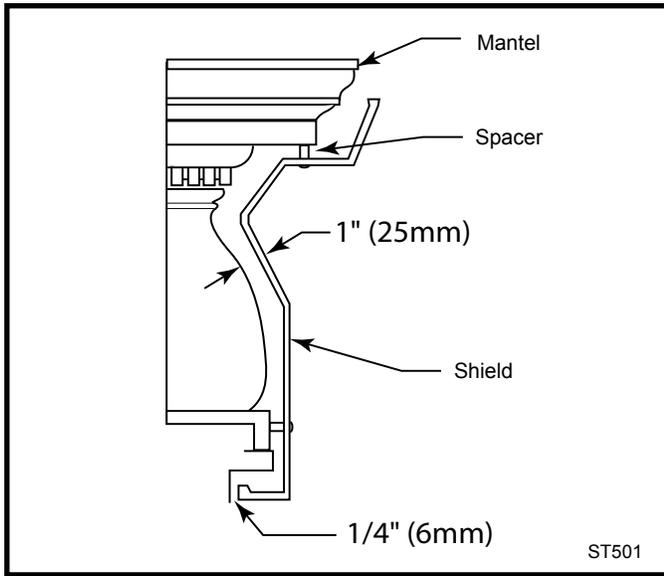
Fig. 14 A custom-formed mantel shield.
