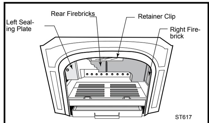
**Fig. 33** Remove left and right sealing plates.
