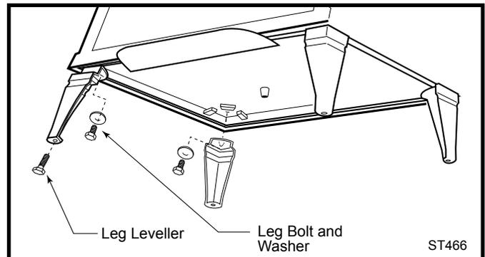
Fig. 26a Attach stove legs and leg levers.
