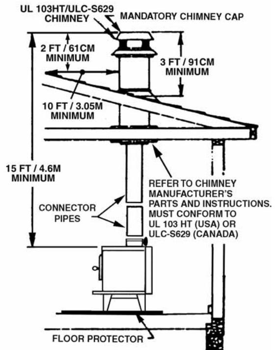
Figure 16 - Chimney Construction through Attic Space
