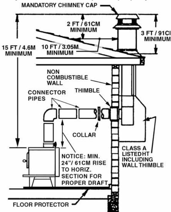
Figure 18 - Chimney Connection to Firebox through Masonry Wall
