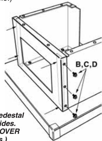
**Figure 4 – Attach Pedestal Front Frame to Sides. (Note– front goes OVER the side panels.)**
