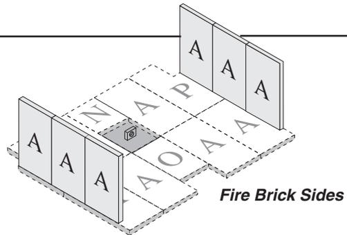
**CAUTION: NEVER OPERATE STOVE WITH MISSING OR CRACKED FIRE BRICKS!**
