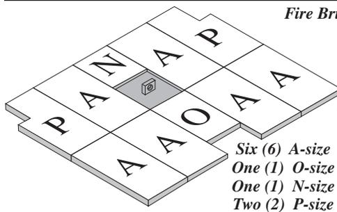
**Figure 13a – Step 1, Bottom Firebrick Arrangement**
