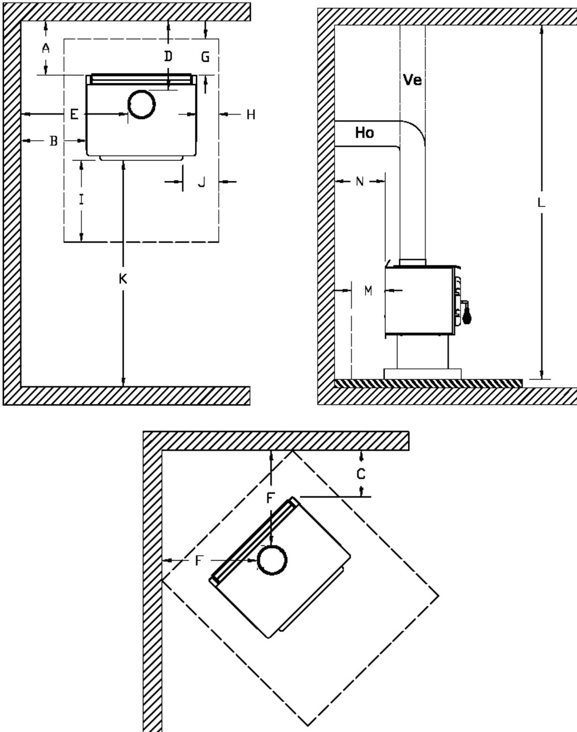
**FIGURE 1.3** Clearances to combustible materials and floor protection
