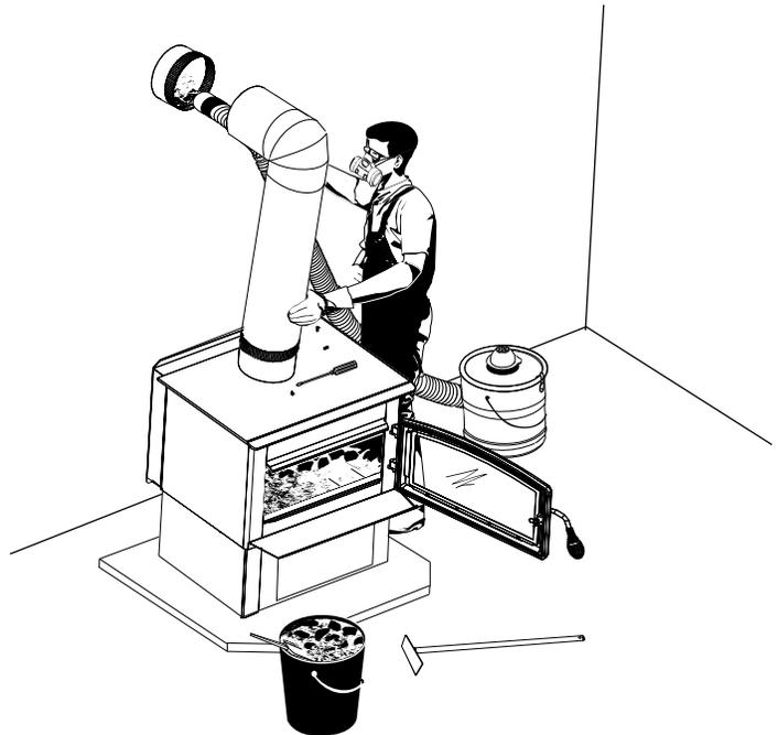
**CAUTION:** Operation of your stove without the baffle may cause unsafe and hazardous temperature conditions and will void the warranty. **NOTE:** Before installing the firebrick, check to ensure that none are broken or damaged in any way. If so, have the damaged ones replaced. Check the firebrick for damage at least annually and replace any broken or damaged ones with new ones. Inspection and cleaning of the chimney is facilitated by the removable baffle.
