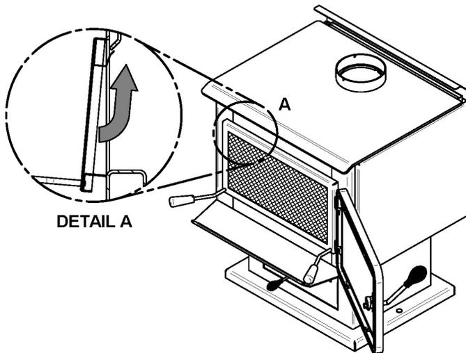
Lean the upper part of the fire screen against the top door opening making sure to insert the top fire screen brackets behind the primary air deflector as in (Detail A).
