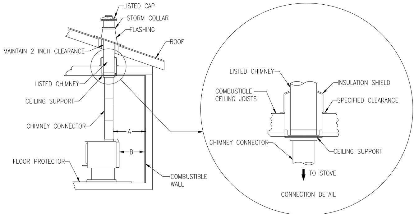
**FIGURE 2.2.1 (B) Typical Installation Through the Ceiling**
